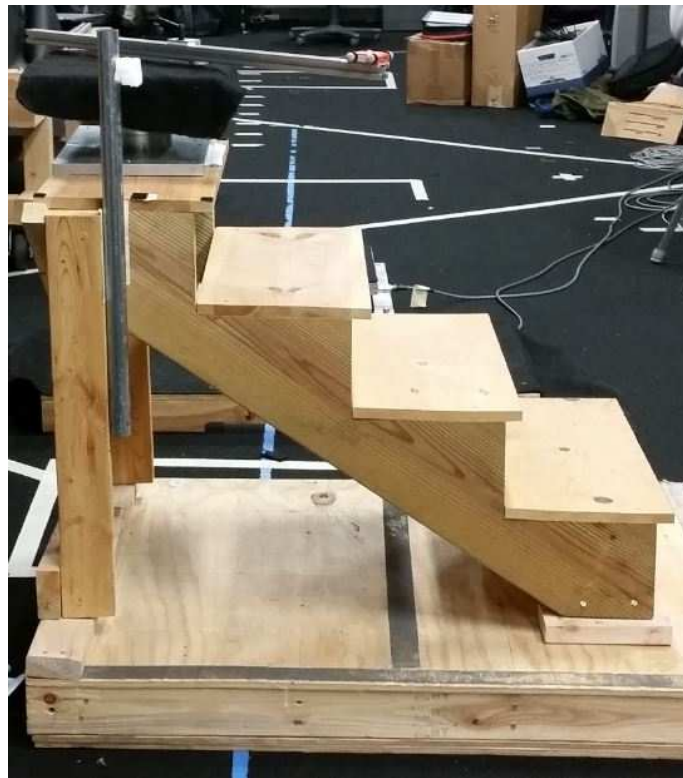
Figure 29: This figure shows the wooden staircase used to sensor apparatus. This provided adequate separation from the ground so as to avoid the disturbance it produced.
